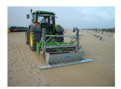
**Big Marlin** is the most widely used beach cleaning machine by professional private traders as well as municipalities in Italy. Equipped with sifting technology for an efficient cleaning of the beach, all the sand is conveyed on the sieve through a plow blade that goes down deep and a front roller provided with teeth that shreds both the sand and the debris.
